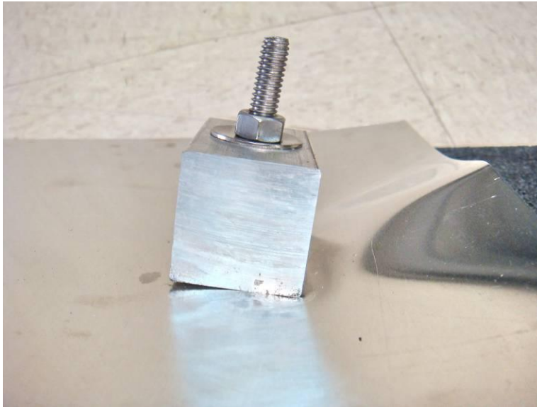
a. Shear Failure
