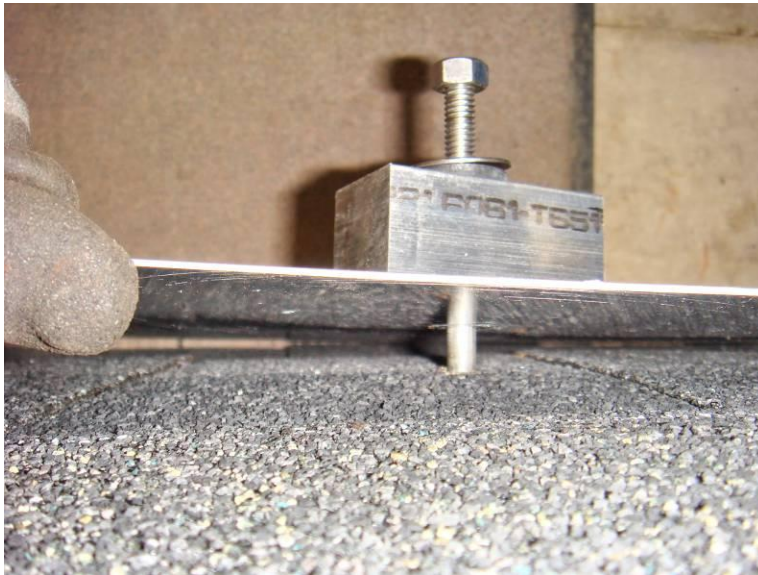
a. Tension Failure
