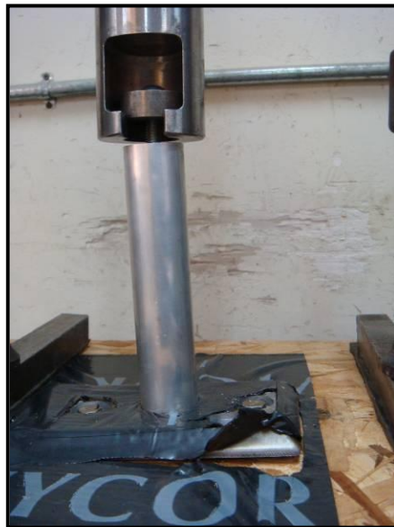
Figure 4. Tensile Test Typical Failure Mode
