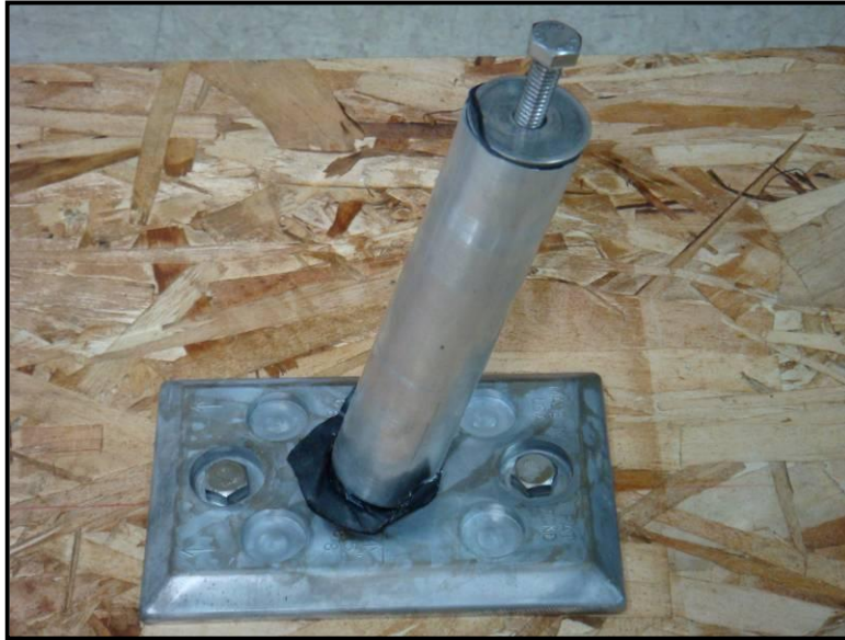
Figure 3. Shear Test Typical Failure Mode
