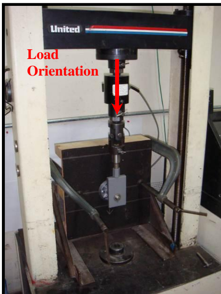
Figure 2a. Shear Perpendicular to Rafter
