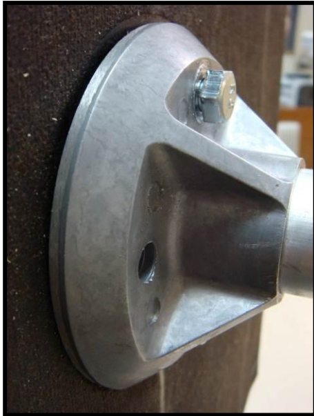
Figure 3. Lag Bolt Pull-Out Shear Parallel to Rafter
