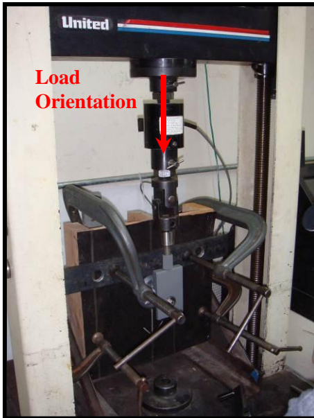
Figure 1a. Shear Parallel to Rafter
