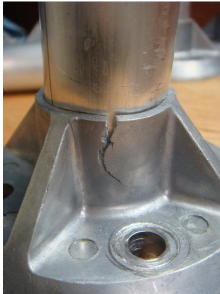
Figure 3. Cracked Aluminum Base Collar Shear Parallel to Rafter
