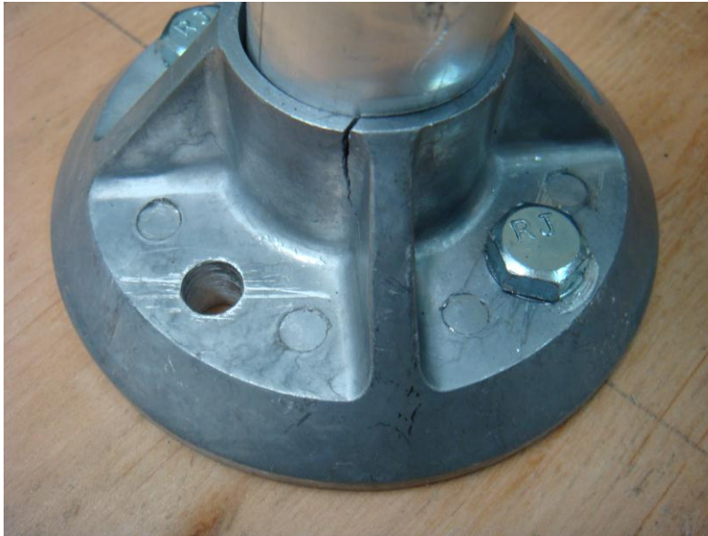
Figure 3. Cracked Aluminum Base Collar Shear Parallel to Rafter
